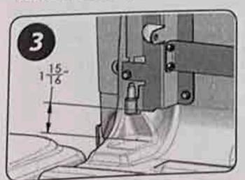
3. INSTALLING MOUNTING BRACKET ASSEMBLY (continued) Mount the bracket approximately 1 15/16" above the floor, according according to the drawing. Using the six (6) self drilling screws provided, attach the bracket to the truck. Be careful not to overtighten and strip out the holes.
