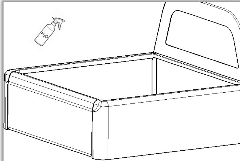
2. Install ① the front/ middle/ rear bracket on ③ side rail, fasten them with ②M6\_16 Hexalobular socket combo with large washer. The way to assembly is same on both sides.
