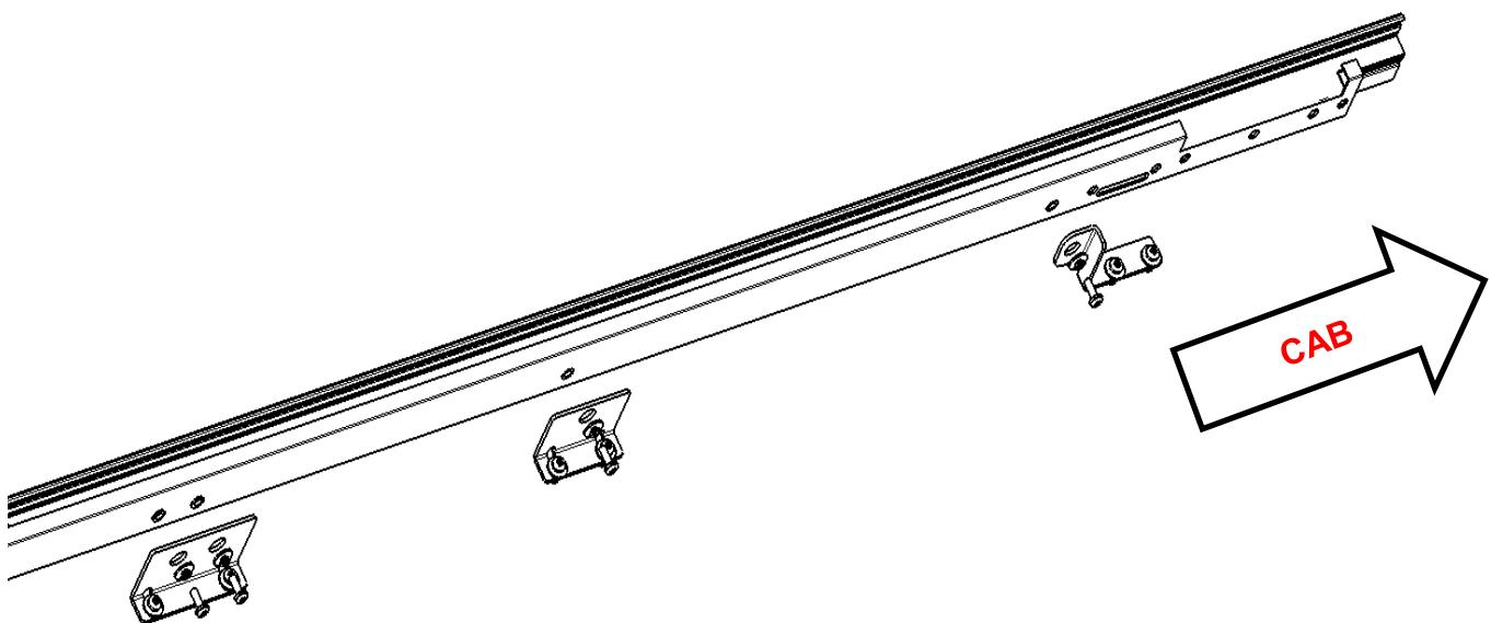
3. Install **(B)** / **(C)** the side rails on **(A)** canister, fasten them with **(3)** Hexalobular socket combo.
