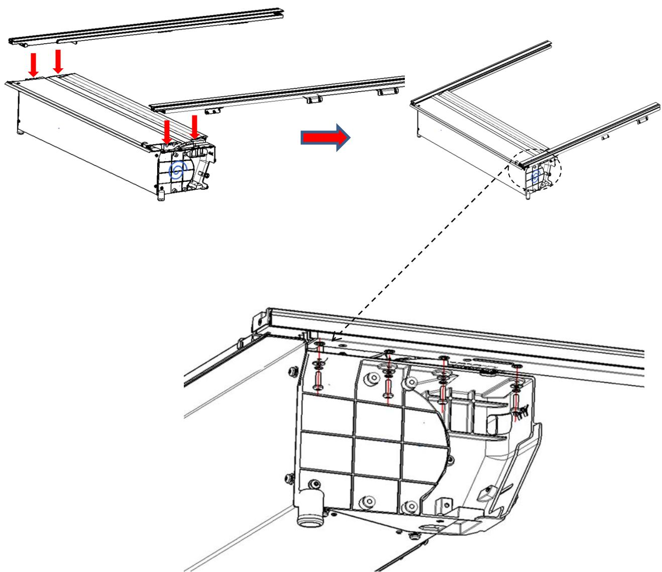
4. Install the front drainage tube on bottom of the canister.
